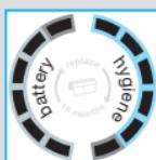
The shaver display ⑯ shows the charge status of the battery on the left, and the hygiene status on the right. (6 dark segments are shown on each side when the battery is fully charged and the shaver is hygienically clean).
