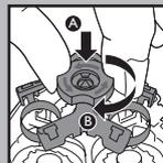
**6** Replace the retaining frame (A) and turn the lock clockwise until it locks into place (B).
