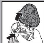
**2** Press the Shaver Head Release Button to open the shaving unit.
