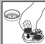
**5** Remove the shaver heads and place the new shaver heads in the shaving unit. Make sure the notches on both sides of the shaving heads fit exactly onto the projections in the shaving head holder
