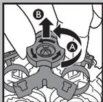
**4** Turn the lock counterclockwise to unlock (A) and remove the retaining frame (B).
