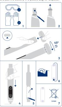
Open the handle as shown, remove the battery and dispose of it according to local environmental regulations.
